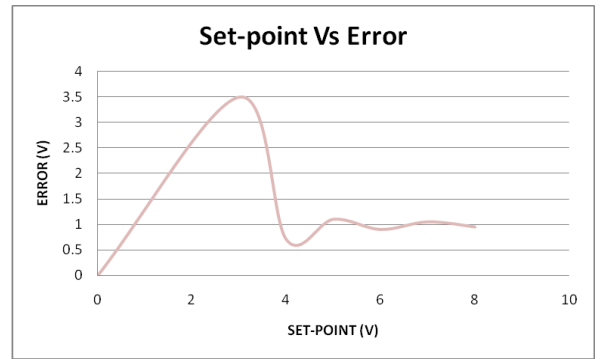
Figure 12: Set-point versus error of PD Controller.
