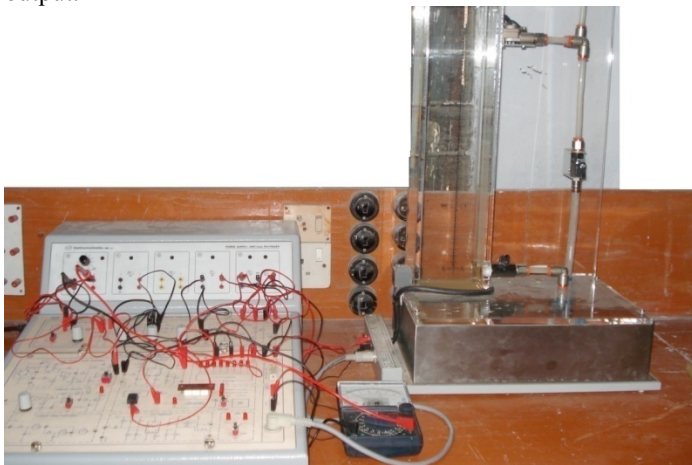
Figure 6: Water tank liquid level control with PID.
